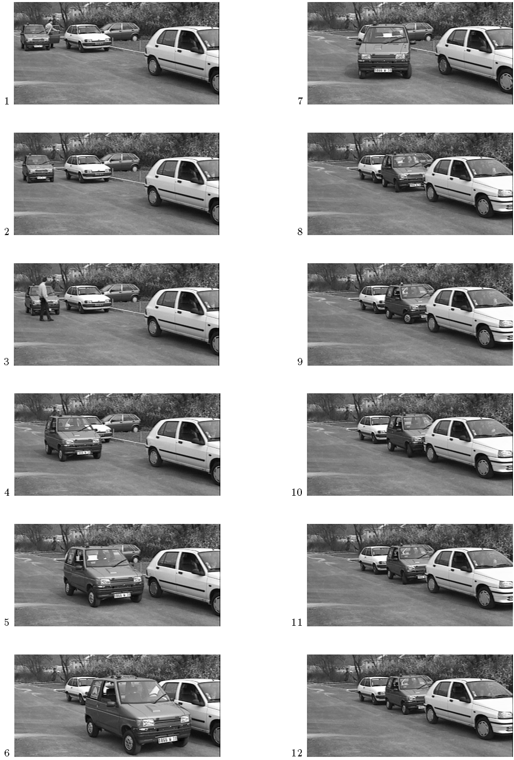
Figure 6: sequence of motions during autonomous parking
