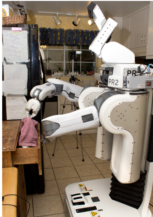
Fig. 1. A mobile robot, operated by a motor-impaired user, performing a manipulation task in a real home environment.
