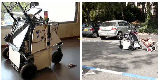
Fig. 9. ANG picking up fallen keys using the actuated pick-up reacher and towing a shopping cart.
