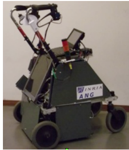
Fig. 8. The Assisted Navigation Guide (ANG walker) [34] is equipped with various sensors and a bistable clutching mechanism
