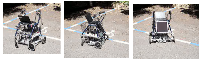
Fig. 7. The sun mode : the walker rotates until the solar panel is perpendicular to the sun and then goes into a sleep mode. After 15 minutes it rotates clockwise until the light measurement is maximum.
