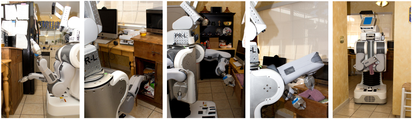
Fig. 12. PR2 robot, operated by a pilot user, performing a mobile manipulation task in the user's home. From left to right: grasping a cabinet handle, pushing open a cabinet door, opening a drawer, grasping a towel inside the drawer, and navigating to desired drop-off location.
