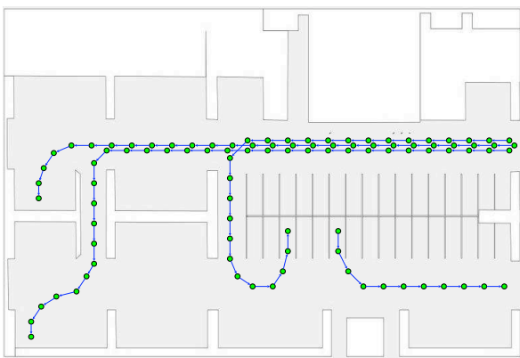
Fig. 14 An HMM structure for a parking environment, where motion patterns are represented as non connected order 2 subgraphs (only a few motion patterns are displayed).
