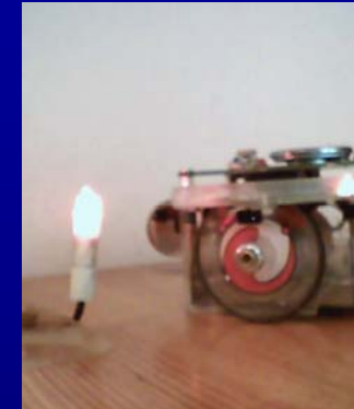
Simultaneous calibration of Odometry & Bearing sensor [Martinelli 08] (Coop. ETH Zurich)
