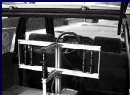
CCD Linear camera + Infrared target (high rate & resolution)
