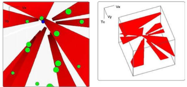
Fig. 1. *NLVO examples* In  $\mathcal{V}$  (left) the green disks represent the obstacles, the blue one is the robot, and the red shapes (one by obstacle) constitute the *NLVO*. The expression of the *NLVO* in  $\mathcal{V} \times \mathcal{T}$  (right) gives an extra information on the time to collision associated with each velocity.
