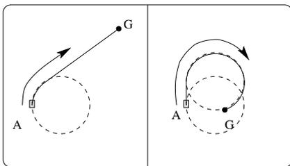
Fig. 2. *Geometrical Paths to the goal* we consider a path composed of a segment of line and an arc of circle. Two cases are possible: The robot turns to align with the goal then go straight in its direction (left). When the goal is inside the minimal circle described by the robot, the robot must go straight first, then turn (right).
