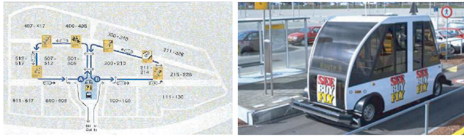
Figure 1 ParkShuttle system within Schipol airport parking lot
